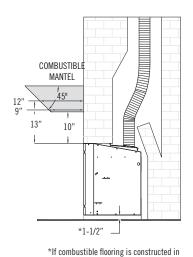
front of the unit, the appliance must be raised 1-1/2" (38mm) using a non-combustible material
