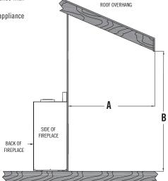
The overhang (A) must be a minimum of 1/2 or greater of the roofline elevation (B) above the base of the fireplace.
