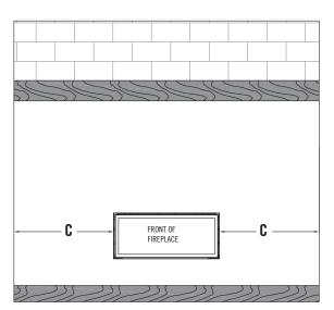
The width of the overhang to each side of the appliance (C) must be a minimum of 1/2 or greater of the roofline elevation (B) above the base of the fireplace.
