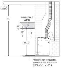
\*If removing existing floor, see manual for floor protection requirements.
